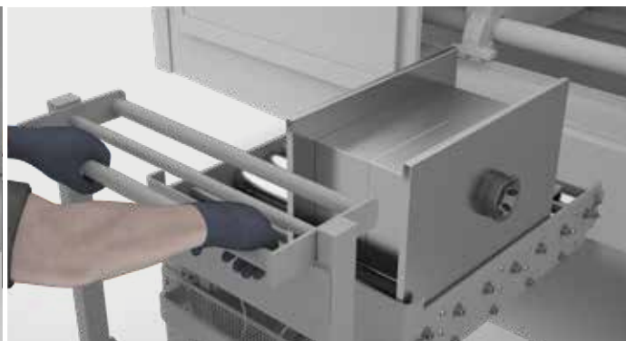
The safety brake system prevents independent movements of the mould loading vehicle.
