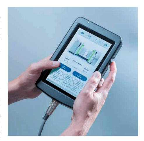
To ensure perfect coordination between the press and its clamping system, the IMAG integrates and displays signals from the machine according to Euromap and SPI AN-145 (mould change mode, MCS available).
