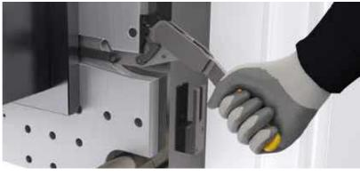
**Mechanical safety lock** When the clamping lever is used the threaded clamping cartridge is automatically mechanically secured.
