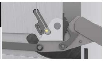
**Safety is maximised with an optional proximity switch** An optional proximity switch can be used to indicate whether the system is in a locked position.
